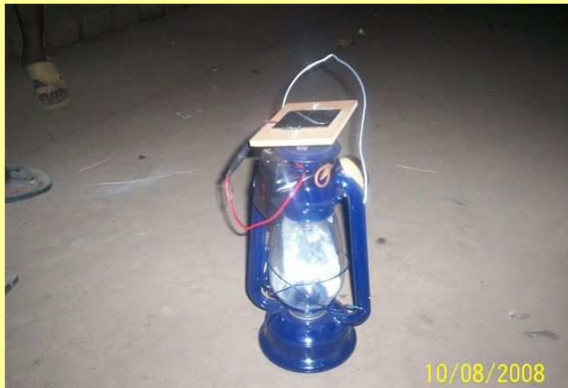
CoBu conducted a simple development of solar lantern using kerosene lantern and diodes, at Malinyi, Tanzania.
